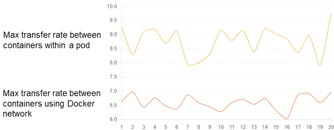
Figure 65 - Containers within a pod have higher bandwidth available than dockers
