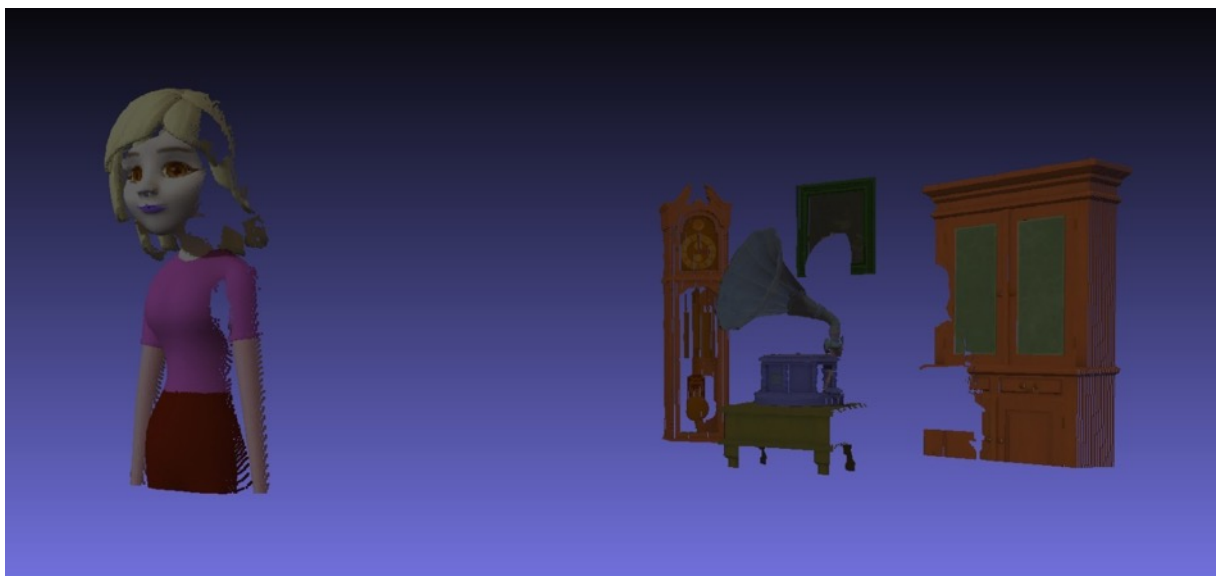
Figure 17 - A test scene reconstructed from 8 RGBD views.
