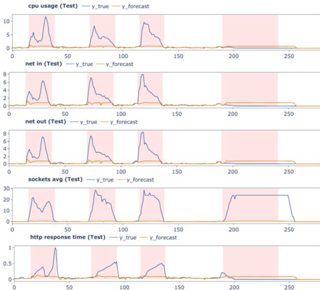
Figure 120: Predictive Analysis of Video Streamer CNF Performance and detection of Hulk and Slowloris attacks in testing data [89].
