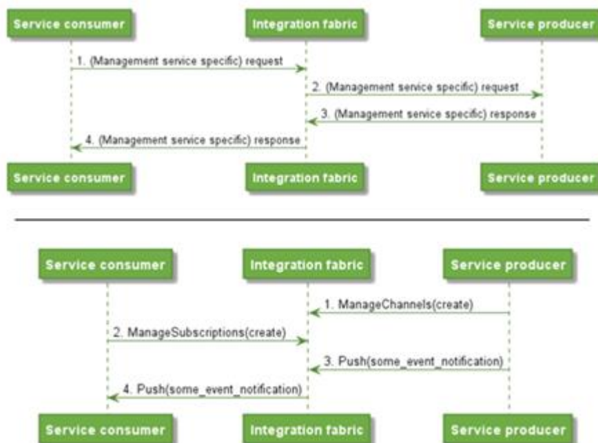
Figure 14: Synchronous Request-response (top) vs Pub/Sub via push (bottom) [43]
