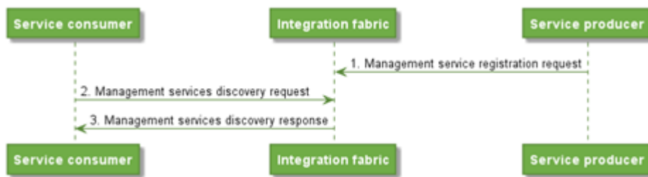
Figure 13: ZSM Service Registration and discovery [43]
